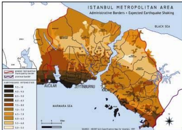
Selected districts in project (Adapted from NEHRP Soil Classification Map for Istanbul 1997)
