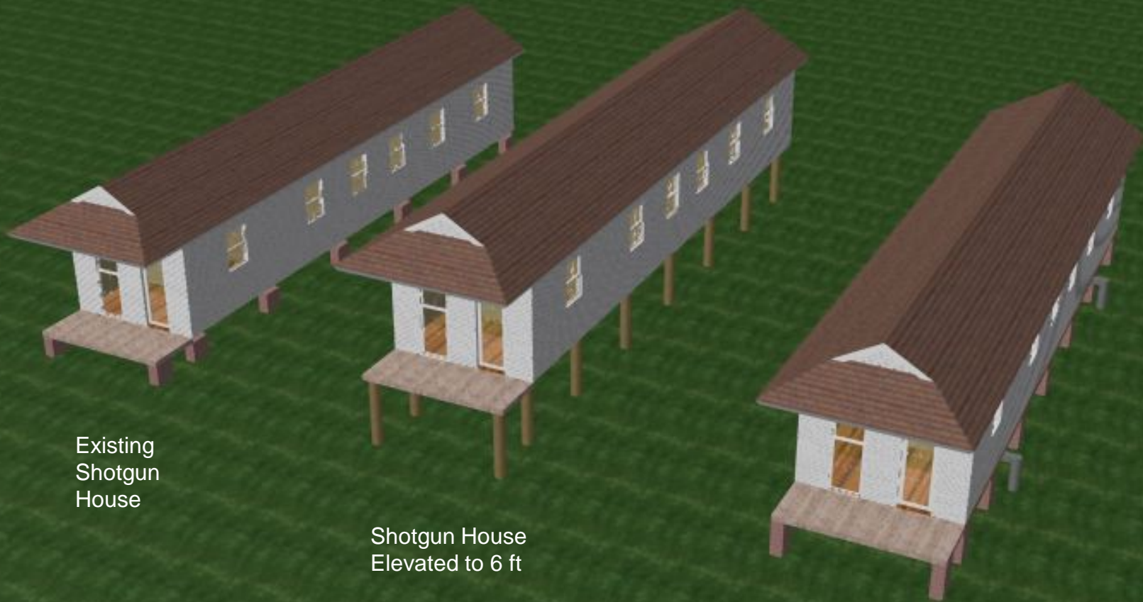
Shotgun House on a Buoyant Foundation
