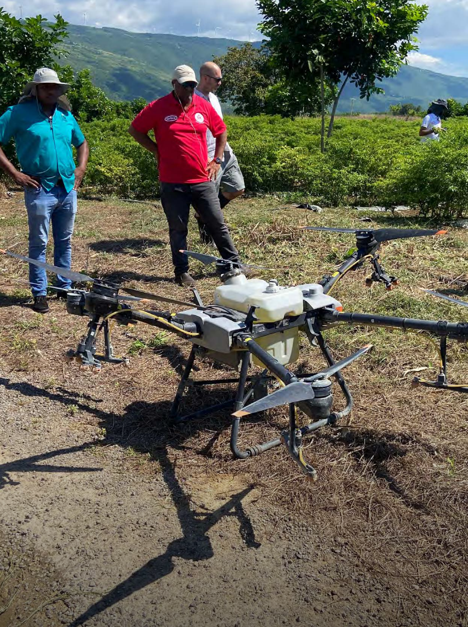
The GAP drone spreads pesticides and water on the fields. In future it will be used to detect pests at an early stage.
