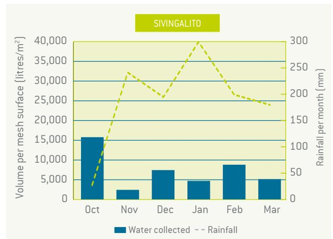
Figures 13, 14, 15 and 16 show the total accumulated volume for each month, measured by the flow meters located at the end of the set of CloudFishers at each site.
