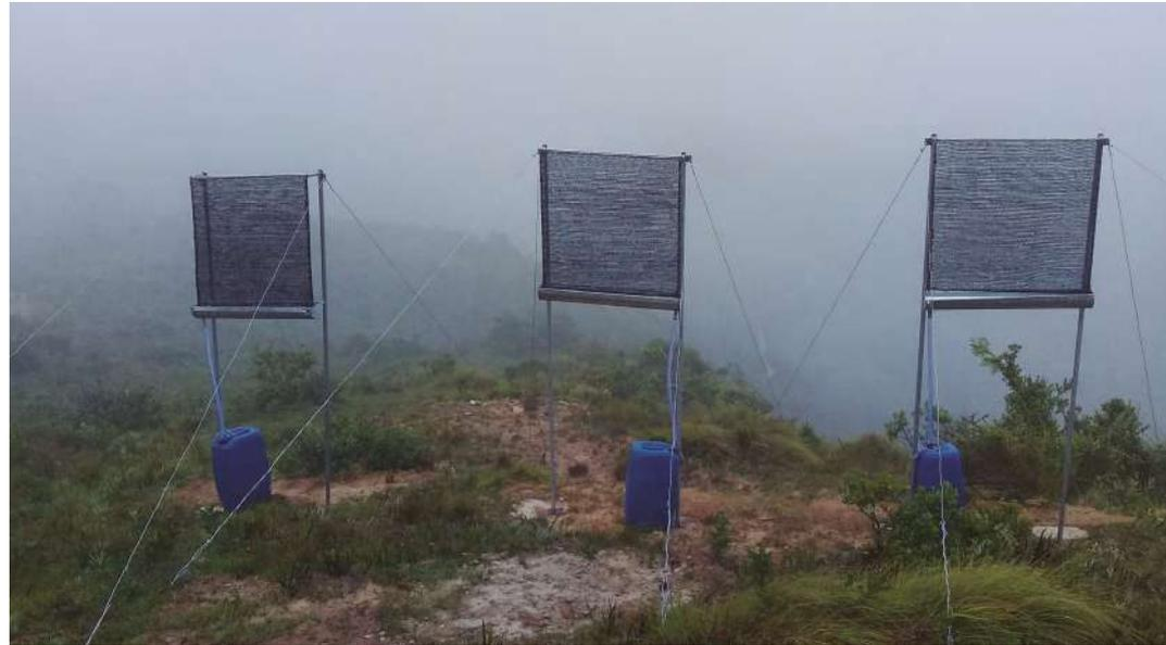
a surface area of 1 square metre, according to the internationally standardised design [Standard Fog Collector<sup>9</sup>], with a Raschel mesh with a 50% shade coefficient. Additionally, weather stations were set up to monitor the weather conditions at each site and the fluctuations throughout the year.
