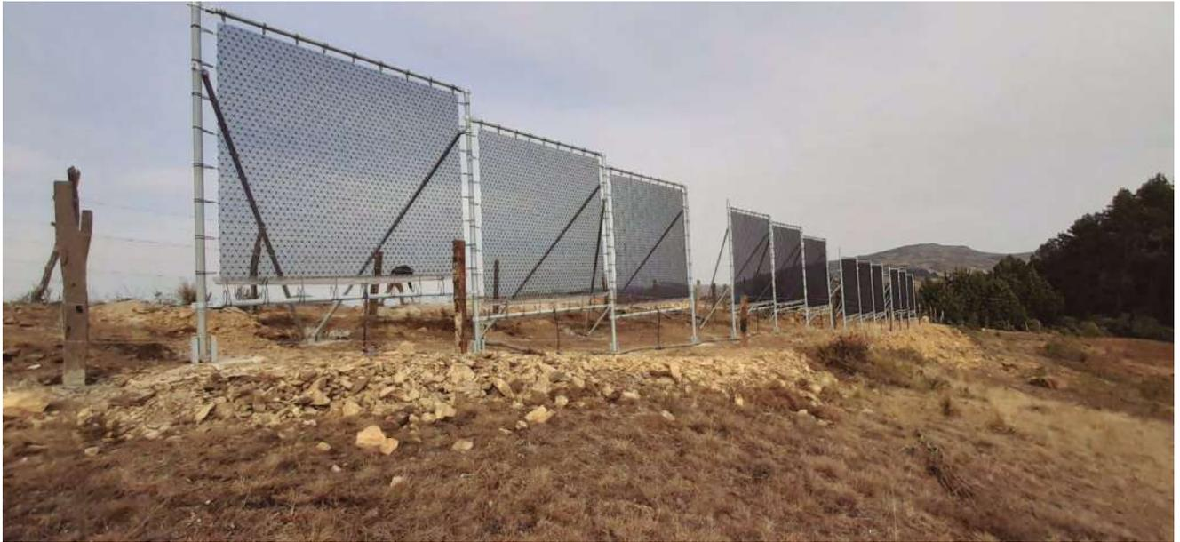
Figure 10. Diagram of the fog collector system at the Sahuintito site
