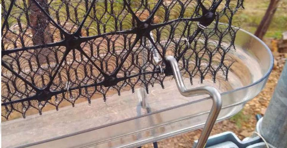
had a larger surface area than the flat mesh. To cross-check the data, the researchers changed the position of each mesh three times, to ensure that the measurements reflected the differences in the quality of the meshes, rather than their location. Following the pilot phase, the first CloudFisher installations were successfully implemented in Morocco and Tanzania.
