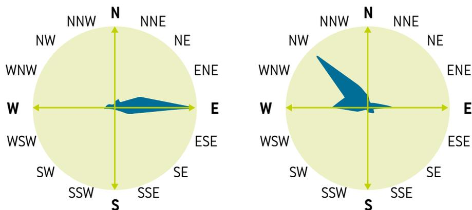
In the case of Sivingalito, for example, the predominant wind direction was NNE and the collectors were positioned at an orientation between 280° NW (the first one) and 320° NW (the last one). In other words, they were oriented virtually perpendicular to the wind, as shown in figure 5.
