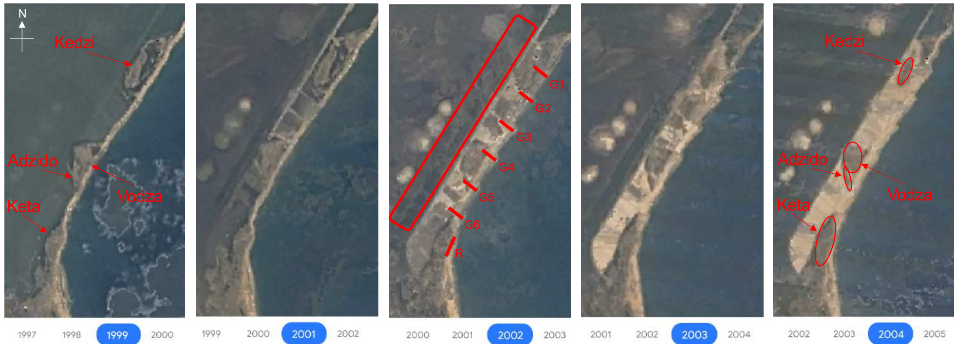
Satellite images of different stages of Keta Sea Defence Project (KSPD), covering the communities of Kedzi, Vodza, Adzido and Keta (from north to south) – before initiation (see 1999 image) and during implementation between 2001 and 2004; KSDP involved a) the construction of a new road at the lagoon side (at half-finished state in 2001 image), b) the construction of a revetment at Fort Prinzenstein in Keta (marked with R in 2002 image) and six groins (marked with G1 - G6 in 2002 image) for halting coastal erosion, and c) pumping of sand from Keta Lagoon (extraction area marked with rectangle in 2002 image) between and to the back of groins to reclaim land from the lagoon and ocean, and to raise the elevation of low-lying portions of already existing land (beige areas indicating both reclaimed and raised land, discernible from 2002 image onwards) and remaining uncovered original land at time of project end (dark brown areas, marked with ovals in 2004 image) (Source of satellite imagery: Google Earth Engine, 2023)
